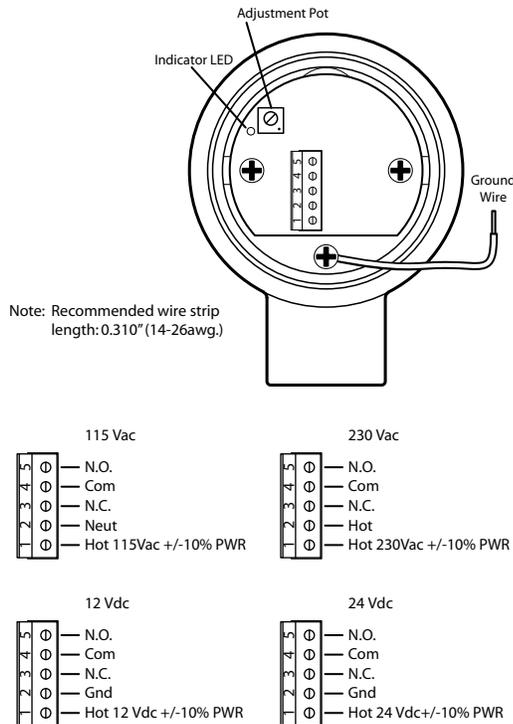
Figure 3: Set Point Adjustment
