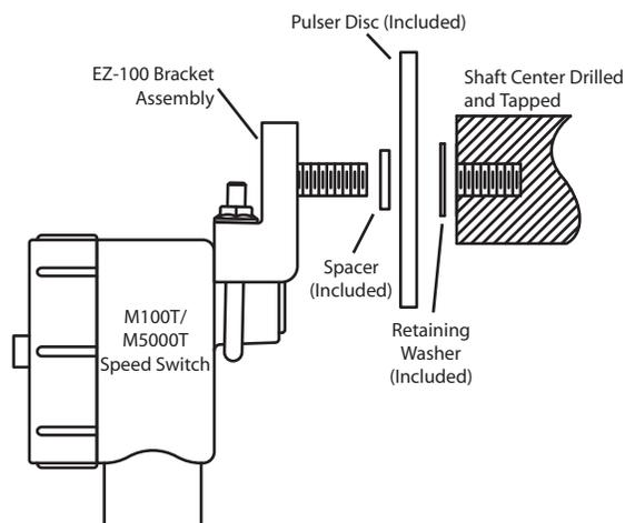
**Figure 8: EZ-Mount Bracket installation**
